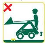
**Figure 6** Operating forward/reverse wheel controls suddenly may cause the loader to behave erratically even on flat ground. On sloping ground, any sudden lifting of one end of the machine may cause it to become unstable or overturn.
