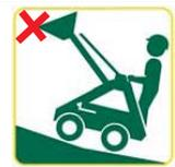
**Figure 4** When moving from a shallow incline to a steeper one (up or down), the operator may underestimate the final angle destabilizing or tipping the loader.
