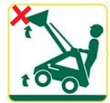
**Figure 8** Sudden stopping of upward bucket movement can make the loader buck and on a slope this movement can be enough to overturn the loader.
