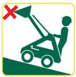
**Figure 1** The weight of an operator may cause the front wheels to lift in some situations. Raising the load on an up-slope transfers the weight of the loader back towards the rear wheels. Raising the load fully and/or the operator on the back may cause the front wheels to lift.
