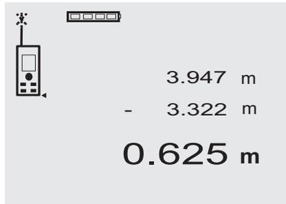
Individual distances can be conveniently subtracted from each other, e.g. in order to determine the distance between the underside of a pipe and the ceiling.
