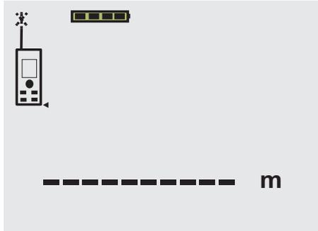
Aim at the target. Press the “Measure” button once again to measure the distance. The result usually appears in the result line in less than a second and the laser beam then switches off.
