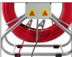
Apply signal from transmitter to both terminals (without using any earthing) to energize leading tip of rodder which then acts like a sonde.
