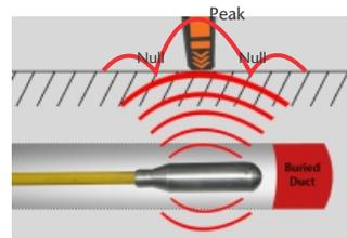
Localize front leading tip of rodder & in turn blockage points with precision using any digital or analog receiver.
