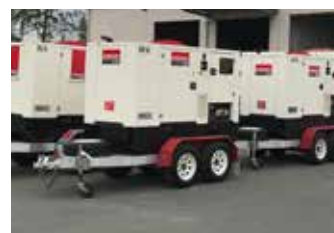
TRAILER MOUNTED GENERATORS
